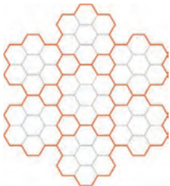
Construction of 7x7 wire rope.
